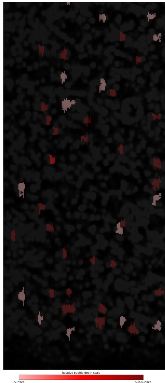
Figure 1.7 A grayscale image of ALHIC1901_228_4-1 with an overlaid color map of various bubbles showing the depth of the bubble as determined by a change in size across channels (.4 \mu m, .6 \mu m, and 1 \mu m).
