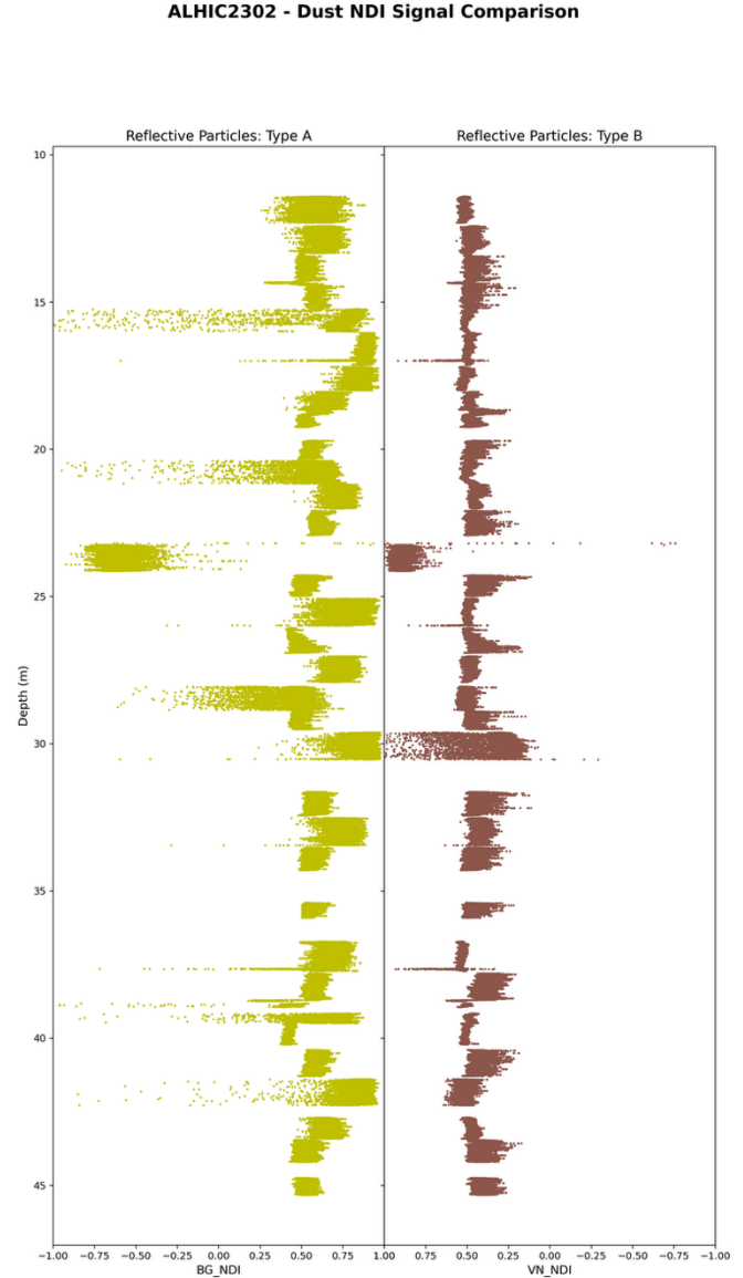
Figure 1.13 This plot depicts the Blue-Green (.42μm and .52μm) Normalized Difference Index in yellow and the Visible-NIR (.52μm and .98μm) Normalized Difference Index in brown. The x-axis for VN-NDI is reversed for a mirrored comparison.
